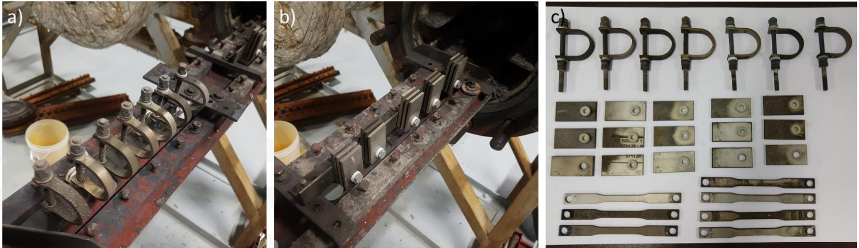
The samples from the Reykjanes testing; a) the U-bend samples, b) the rest of the samples and c) all the samples after they were removed from the holders.
