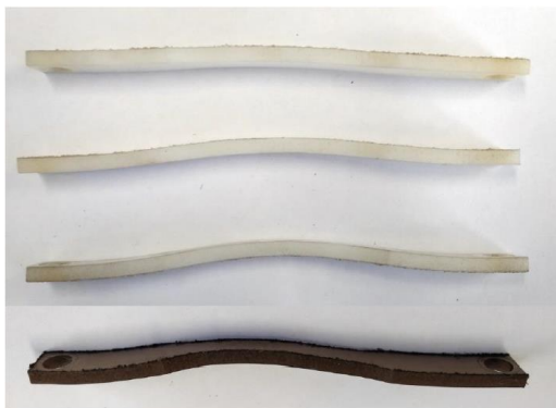
Warping of plastic samples after testing.
